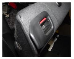
To release both the 60% and 40% backrests from their stationary position simply press the release handle on each side of the backrest before pushing them forward.
