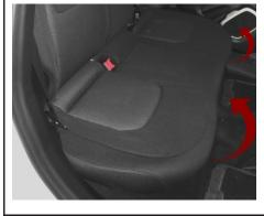
In this final step some force is necessary to remove the seat bottom from its stationary position which is held in place by two forward alignment inserts as illustrated in the next step These alignment inserts simply snap on and off. There is no releaser.
