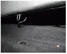
Step into your vehicle and grab the seat bottom from underneath the front edge and pull up until the seat bottom snaps out of place. Once the forward alignment inserts are revealed you can securely remove the seat bottom.
